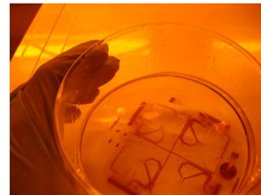
Etch Cr layer using same pattern
